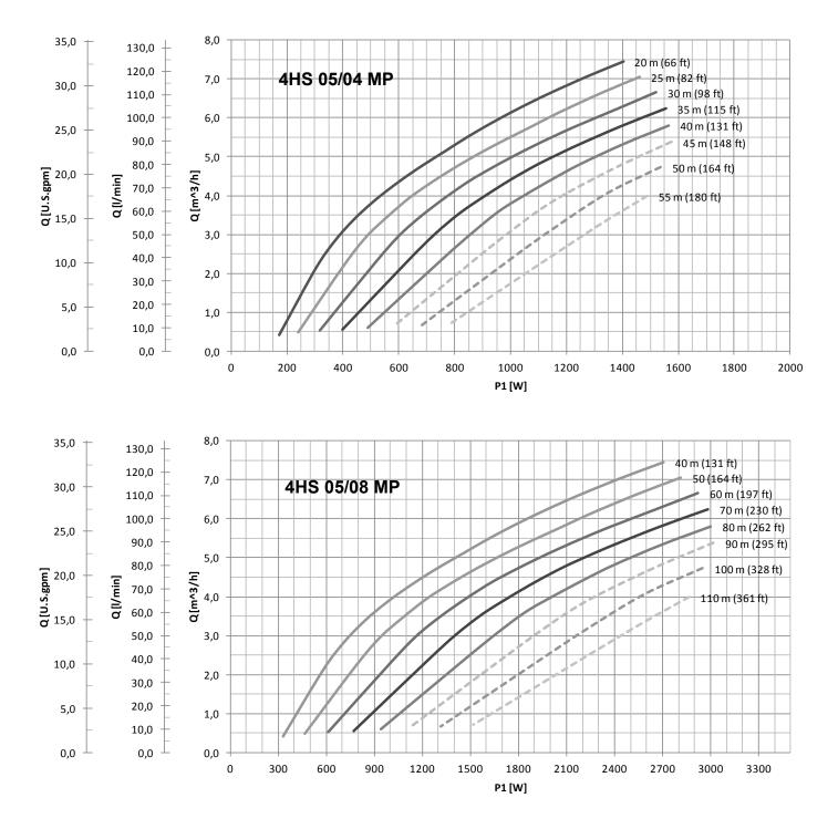
CM MultiPower installation is recommended on dashed lines operation.
