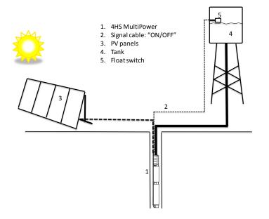
If the CM MultiPower control module is not used, signal cables can be used to control pump ON/OFF the connecting, for example, a float switch.
